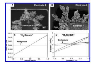
**Figure 1.** SEM images of (A)  $H_2$  sensor device and (B)  $H_2$  switch device and corresponding i-V curves in (C) and (D), respectively.
