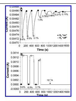
Figure 2. Current-time plots of (A) "H $_2$  sensor" device and (B) "H $_2$ switch" (10 cycles of phenol) measured at -0.3 V in the presence of N<sub>2</sub> initially and of various concentrations of H2 (H2 on) and 100% N2 (H2 off) as indicated.
